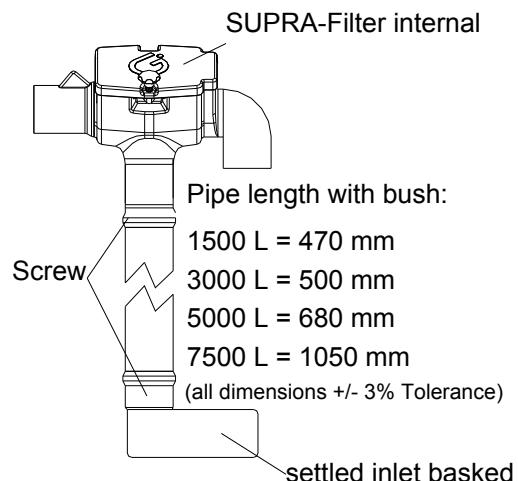
Following this a 250 mm long inlet pipe and an overflow siphon are pushed in to the Li-Lo underground tank until the end stop position as shown in the adjacent depiction.
