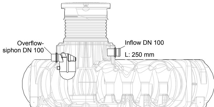
Now the prepared SUPRA®-Filter internal is installed in the tank, the elbow of the overflow from the filter is also connected now to the siphon. The inlet pipe is so to position that it is flush with the filter inlet and then finally fixed in place with the quick assembly collar.
