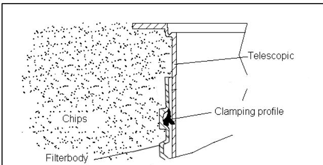
**Attention:** If the lubricating soap becomes dry and the telescope becomes difficult to move then there is the danger that the sealing ring will be forced out of its recess. Before filling the sealing ring must be checked once again that it is seated correctly in position. The telescope must be sufficiently embedded and supported that no forces are transferred to the housing.
